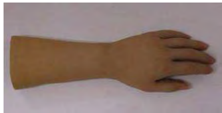
Figure 2.23: Design of 5 D.O.F Robot Hand with an Artificial Skin for an Android Robot [25]
