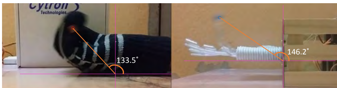
Figure 4.8: The angle of the human pinky finger and the animatronic hand pinky when started to bend
