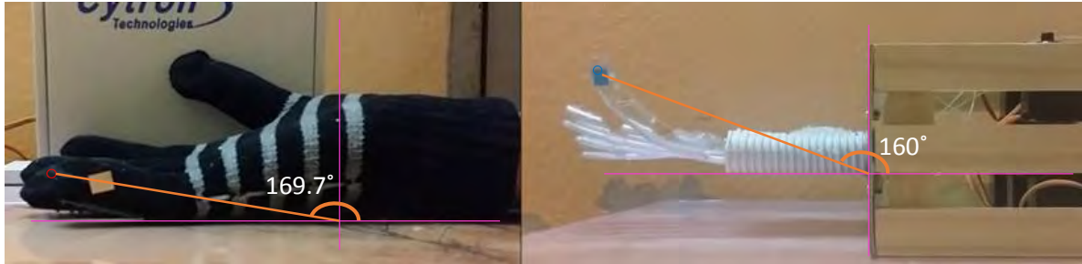
Figure 4.10: The angle of the human pinky finger and the animatronic hand pinky finger in relaxed mode (end)
