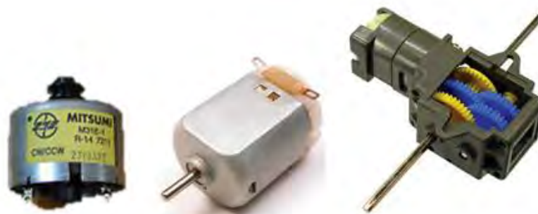
Figure 3.7: Mitsumi M31E-1, FC-130SA-2270, Tamiya #70168 double gearbox. [15, 16, 17]
