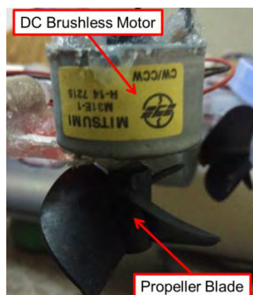
Figure 3.5: Mitsumi M31E-1 DC Brushless Motor with 3.9mm Propeller Blade
