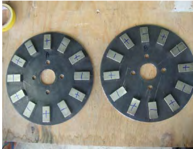
Figure 2.1: Figure: Rotors of Flux Permanent Magnet Generator. (P. Wannakarn and T. Tanmaneeprasert et al.,2011)
