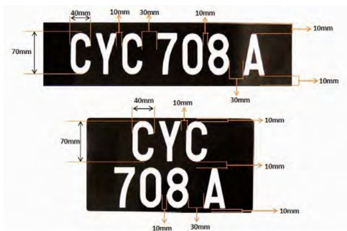
Figure 2.3: The standard measurement of the Malaysian vehicle license plate
