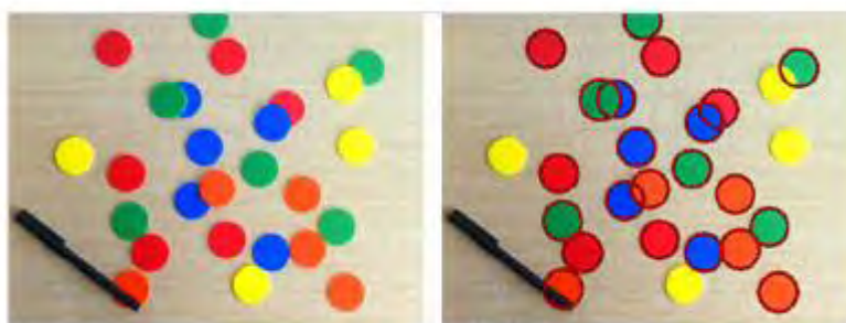
Figure 2.5: The example of image processing using MATLAB for counting circular objects in an image
