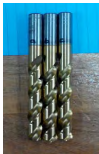
Figure 3.5 : High Speed Steel coated with Titanium Carbon Nitrate
