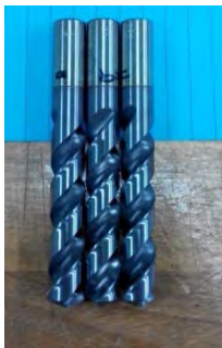
Figure 3.4: High Speed Steel coated with Titanium Nitrate
