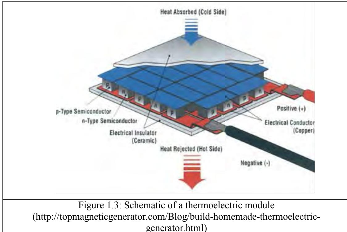
When heat is applied to one surface of the thermoelectric generator, the electrons in the n-type semiconductor and the holes in the p-type semiconductor
