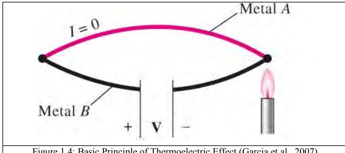
The Seebeck effect forms the basis of the development of thermoelectric generator.
