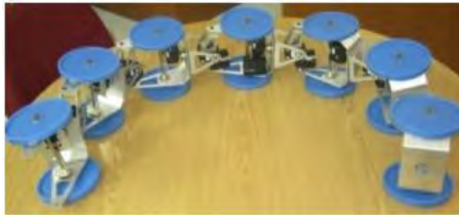
Figure 2.3: The prototype wheel-based modular snake robot. (P. Polchankajorn and T. Maneewarn, 2011)
