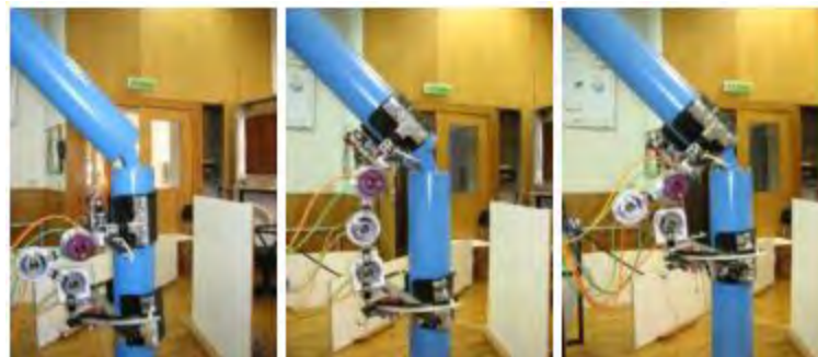
Figure 2.2: The design and climbing mechanism of 3D Climber.
