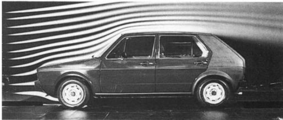
Figure 2.3 : Streamtubes flowing over an aerodynamic body (Wolf-Heinrich Hucho)
