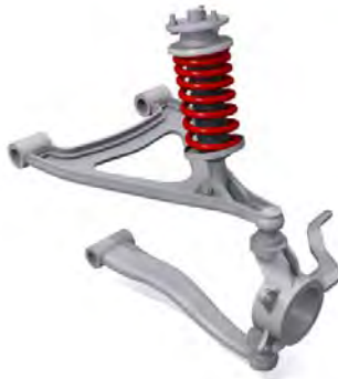
Figure 2.1: A First Type Coil Spring Is Mount (Güler, 2006).
