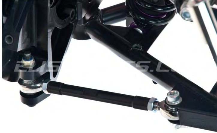
Figure 2.8: Toe Link Position in Double Wishbone Suspension ( www.eliseparts.com ).
