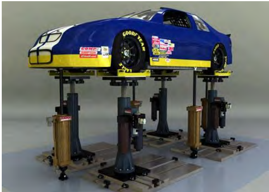
Figure 2.1: Image of 7-post test rig with NASCAR race car
