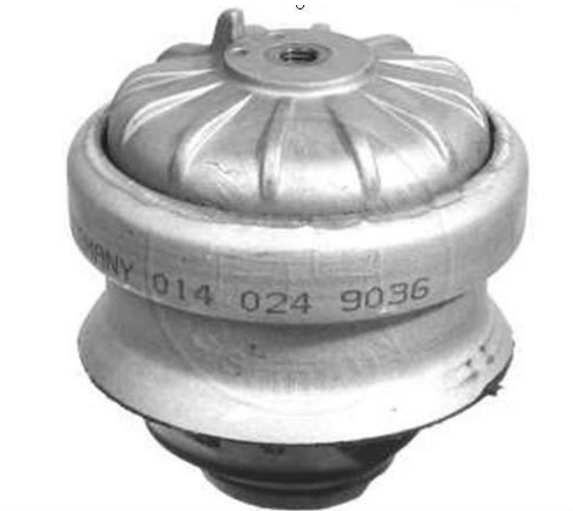
Figure 2.2 (c) : Hydraulic edition of semi-active engine mount type(J. Vinolas, 2009)
