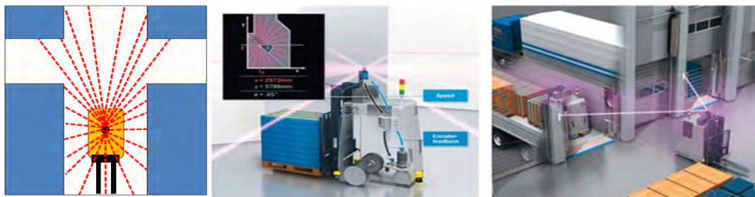
Figure 1.7 : Natural features (natural targeting) ( http://www.mhi.org/agvs )
