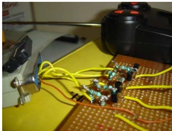
Figure 2.3: Connections between transistor circuit and parallel port
