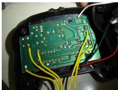
Figure 2.1: Connections of wires at the controller
