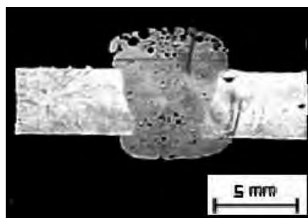
Figure 4.2 Condition 190 A, 19 v, 15 mm/min. Depth of Penetration = 6.46 mm
