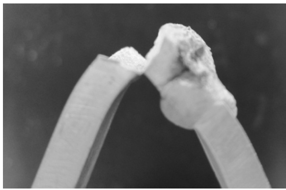
Figure 4.6 The cross section showed a certain amount of pores
