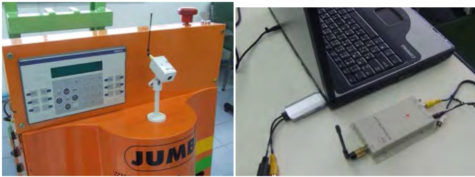
Figure 2.5: Integrated Camera to AGV: a). Wireless Camera Installation, and b). AV-receiver Module in Remote Site of Operation.
