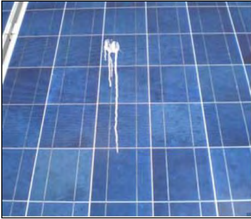
Figure 2.3: The Surrounding Plant and Guano Shading Phenomenon
