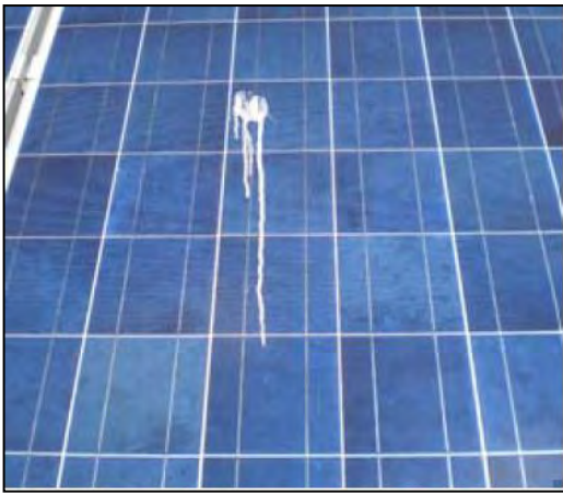
Figure 2.3: The Surrounding Plant and Guano Shading Phenomenon
