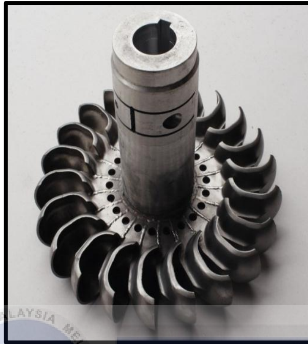
Figure 3.4: Pelton turbine with its shaft
