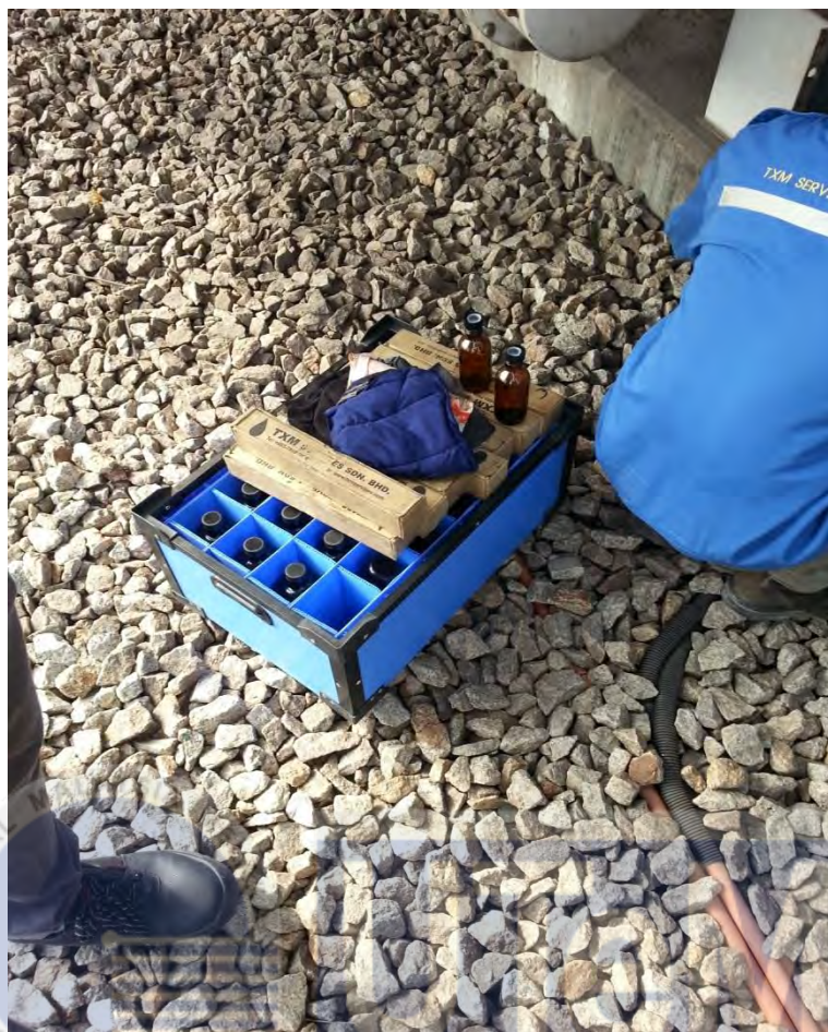
Figure 3.3: Specially Designed Beaker Used to Store the Collected Oil Sample
