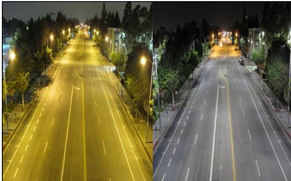
Figure 2.2: The different lighting between HPSV lamp and LED lamp [16]
