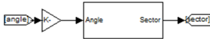
Figure 3.14: Angle to sector calculation block
