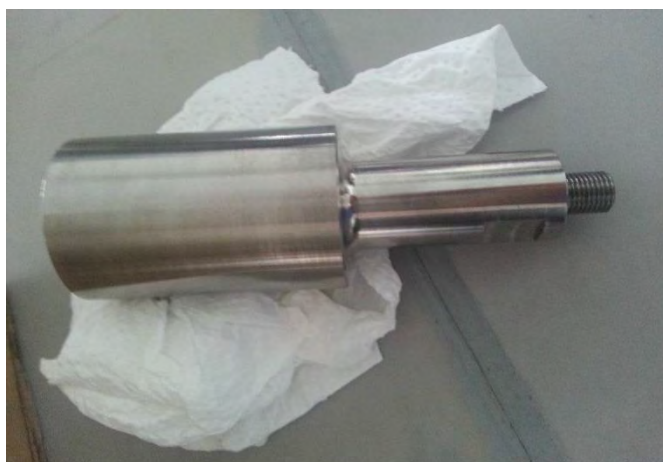
Figure 3.6: 40mm probes made of Titanium
