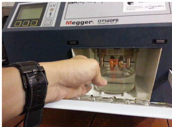
Figure 3.13: The placed of the sample in the test vessel
