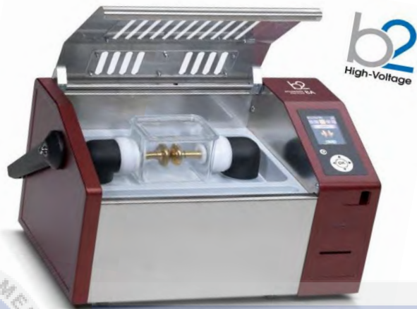
Figure 2.3: BDV testing instrument [13]
