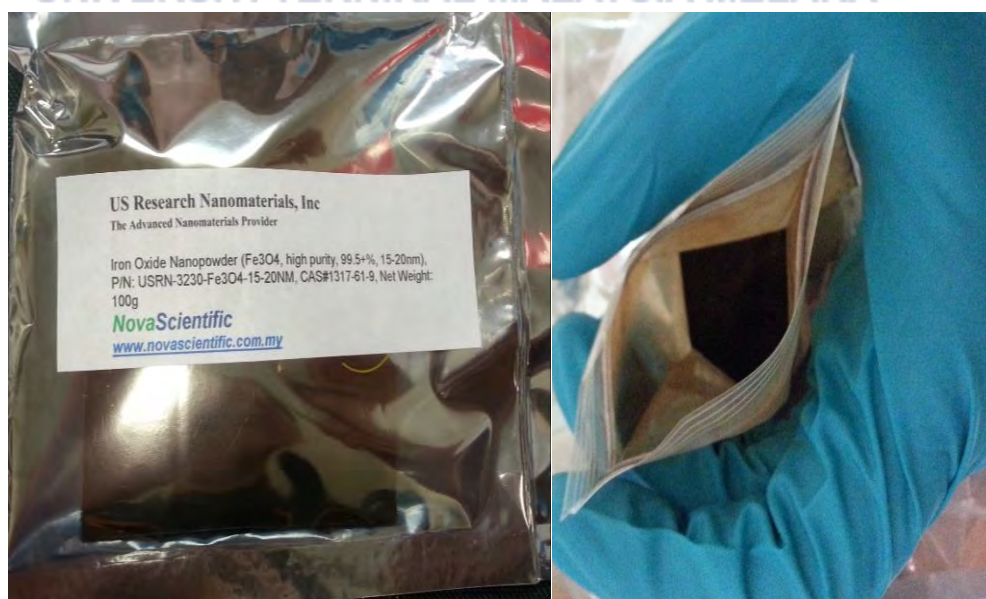
Figure 3.3: Iron Oxide Nanopowder, \text{Fe}_3\text{O}_4
