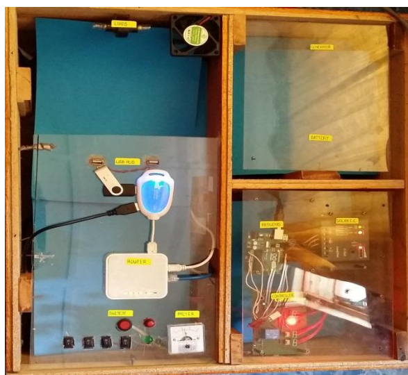
Figure 4.9: Hardware Setup Implementation
