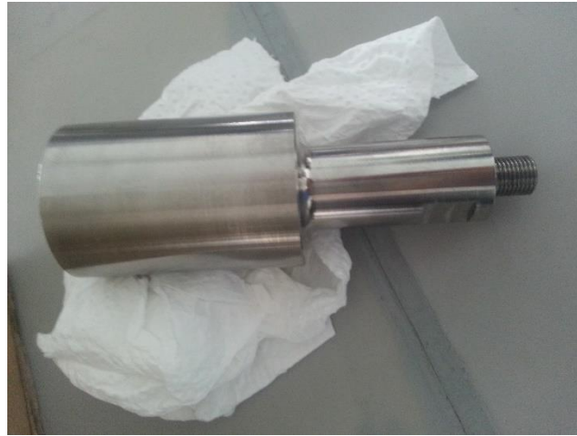
Figure 3. 11: Probe diameter 40 mm, approx., 100 mm long.
