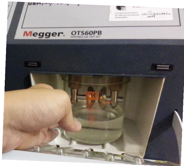
Figure 3. 23: Loading the test vessel.
