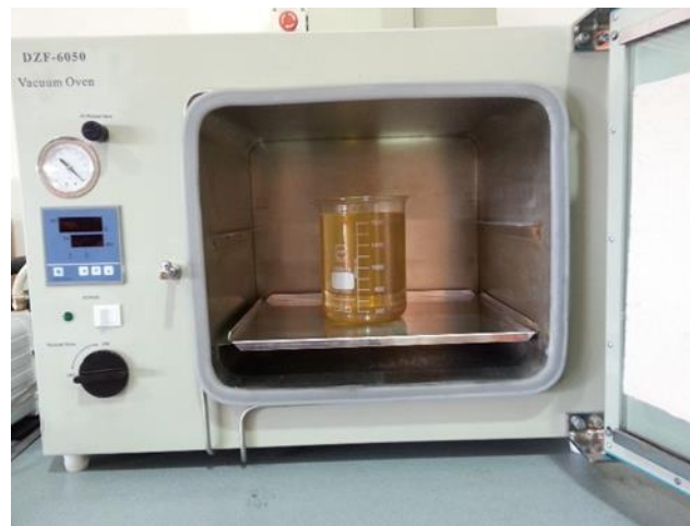
Figure 3. 13: Vacuum drying Oven Process.
