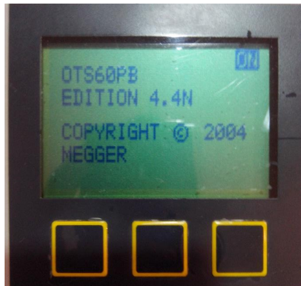
Figure 3. 24: Switch ON the oil test set.
