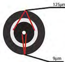
Figure 2.3: Diameter of single mode fiber.
