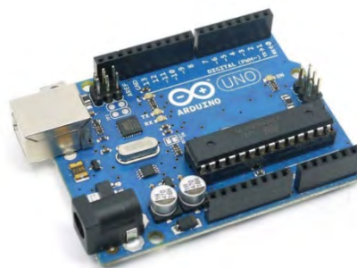
Figure 2.3: Uno board courtesy of [23]
