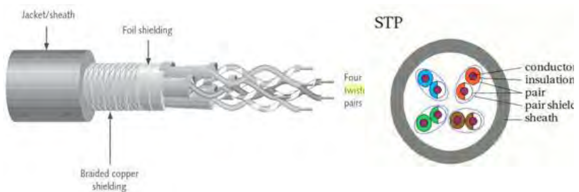
Figure 2.3: Shielded Twisted Pair (STP)
