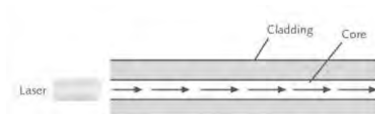
Figure 2.5: Transmission over single mode fiber optic cable
