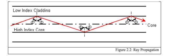
Acceptance angle is the maximum angle at which light may enter the fiber in order to be propagated and is denoted by  $\theta a$  in figure 2.2. The relationship between the acceptance angle and the refractive indices of the three media involved-core, cladding and air, leads to the definition of Numerical Aperture which is given by –
