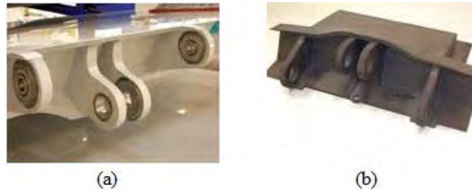
Figure 1.2 : FACC Carbon Composite Center Hinge Fitting (Dawson, 2006): (a) Metal Bushings and Bearings Installed in the Fitting Lugs; (b) Hinge Fitting Molded via RTM
