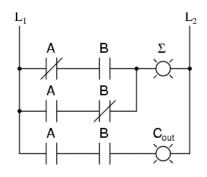
Figure 2.2.1 (a) - Example of simple ladder diagram.
