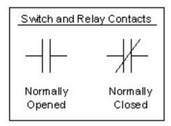
Figure 2.2.1 (b) - The normally open and normally closed contact for ladder diagram.
