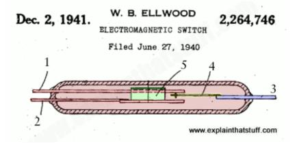
Figure 2.4.1 (a) - The patented reed switch by W.B. Elwood.
