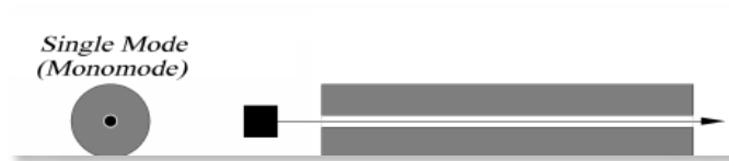
Figure 2.4: Single Mode Fiber
