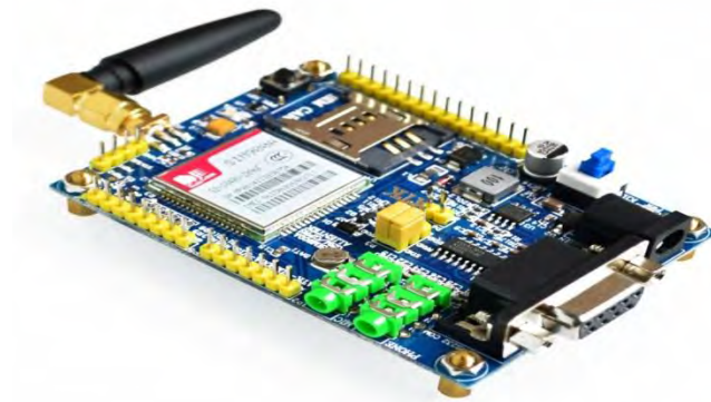
Figure 1.1: GSM Module SIM900A
