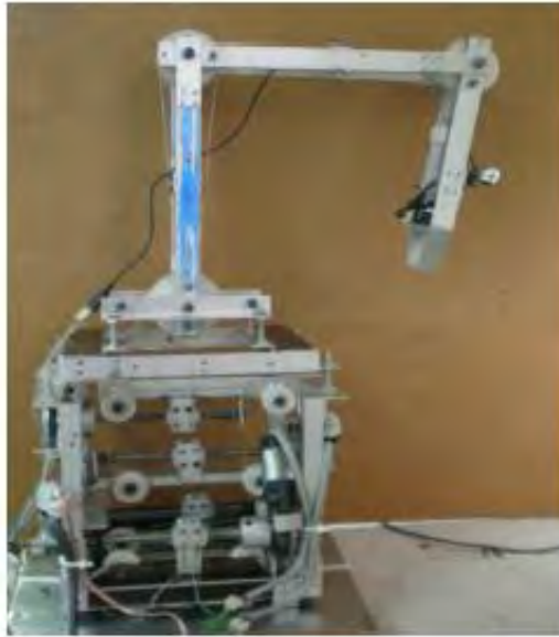
Figure 2.2: Robotic Arm with image Processing
