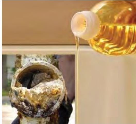
Figure 2.2 : Blockage Pipe due to Cooking Oil
