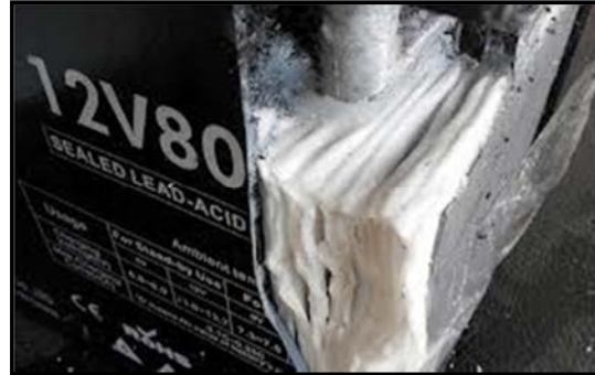
Figure 2. 4: AGM (The Absorbed Glass Matt)
