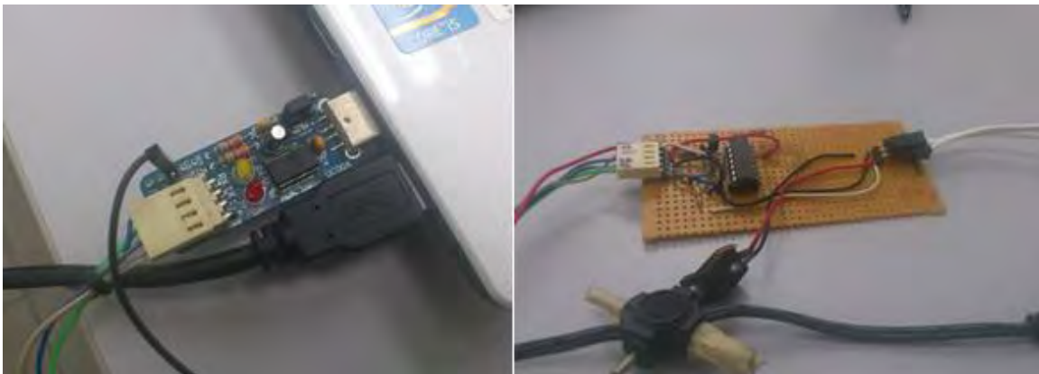
Fig. 9: UART converter and main controller for servo cube G15.
