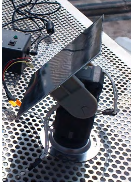
Fig. 8: Heliostat model by using coupled servo cube G15.
