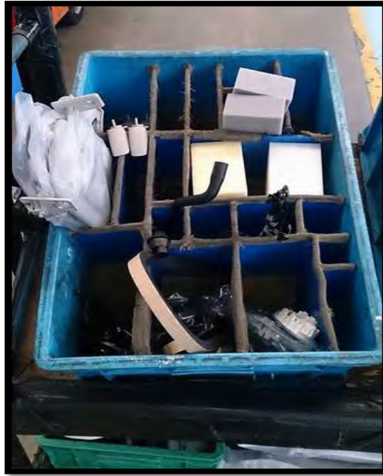
Figure 2.2: An example of kit pallet (Tan Chong Motor Assemblies Sdn Bhd, 2014)
