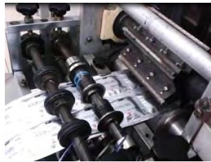
Figure 1.5: Perforated and trimmed equipment (Mohamad, 2014)
