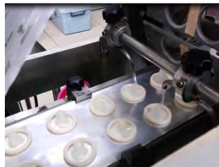
Figure 1.3: Silicone oil being pump on the condom (Mohamad, 2014)
