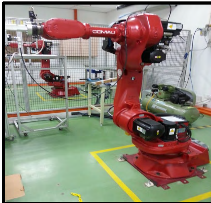
Figure 2.1: SMART NS 10-1.65, COMAU Articulated robot (Source: Image taken from Robotic Lab, at FKP Block B)
