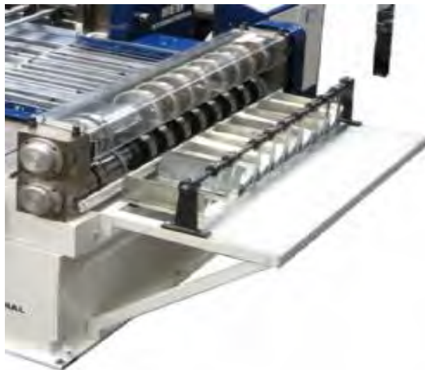
Figure 2.3: The metal strip collector in Comfish Industries Sdn. Bhd. (Comfish Industries Sdn. Bhd., 2014)
