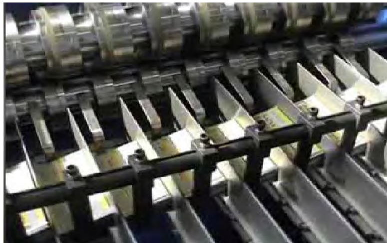
Figure 1.1: The type of double slitting machine collector in Comfish Industries Sdn. Bhd. (Comfish Industries Sdn. Bhd., 2014)
