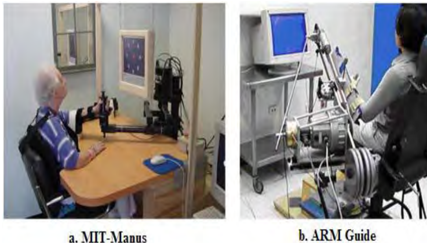
Figure 2.2: Robotic Devices for Arm Rehabilitation
