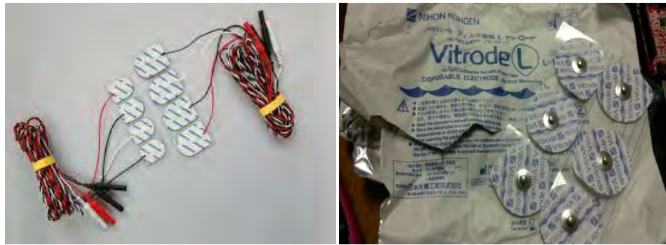
Figure 2.1: Disposable Ag/AgCl electrodes and the active surface electrode
