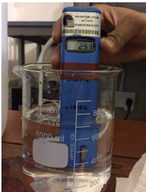
Figure 3.8 : Contaminant With Conductivity of 2.53 mS/cm
