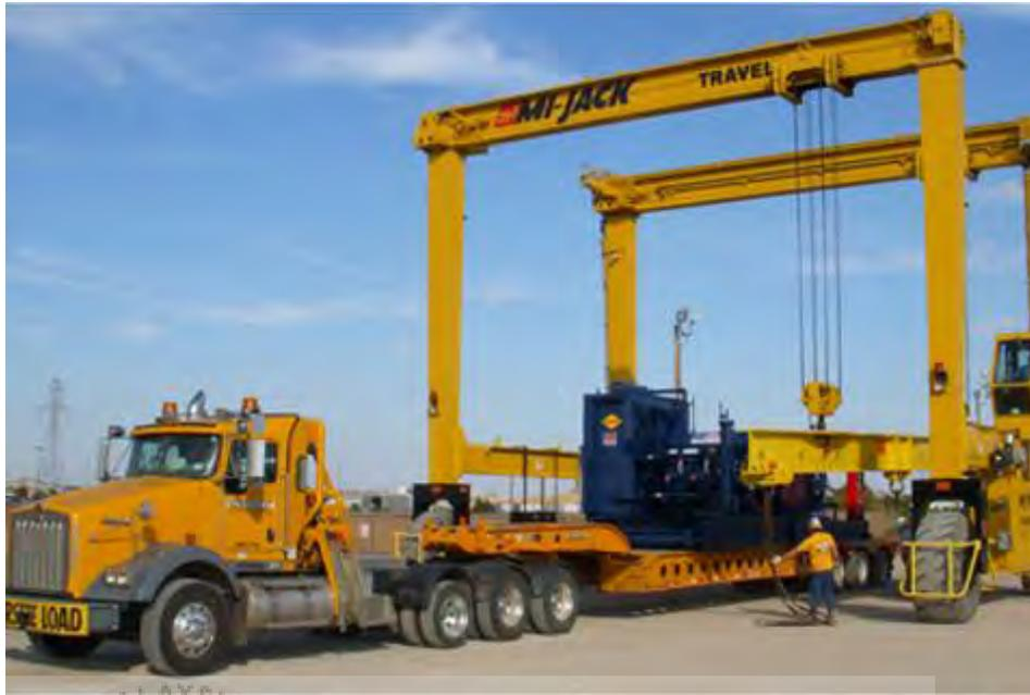
Figure 1.1: Example of a Gantry Crane System
