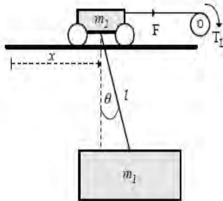
Figure 3.2: Schematic diagram of a GCS [6]
