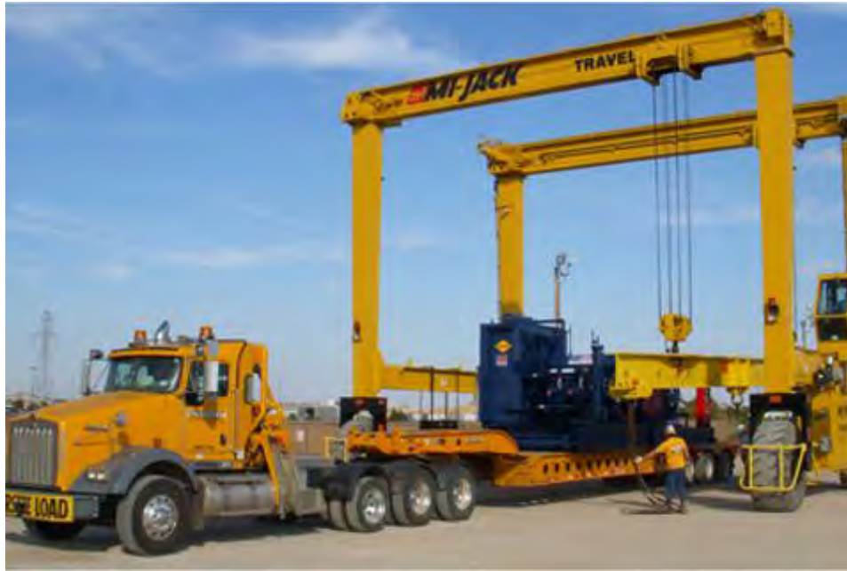
Figure 1.1: Example of a Gantry Crane System
