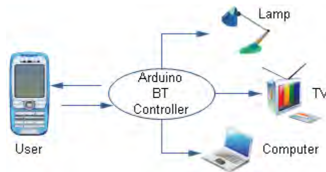
Figure 2.5.1.2: Block diagram of Bluetooth-Based Home Automation System
