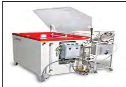
Figure 2.1 : Example of salt fog tested chamber[29]
