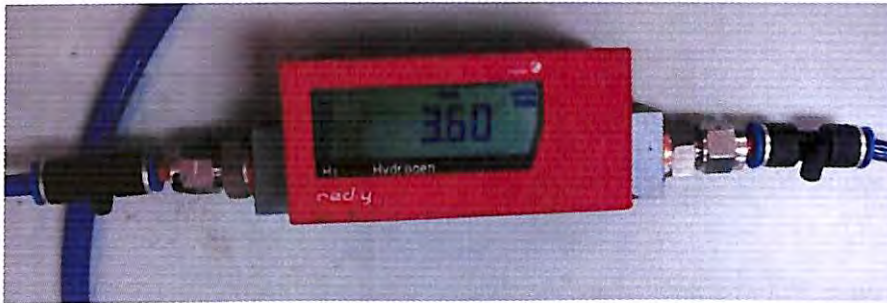
Figure 3.5: Digital hydrogen flow rate meter
